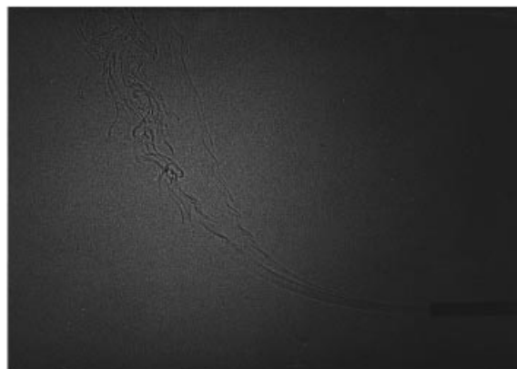
FIGURE 7. Shadowgraph picture of a bifurcating jet at Gr^{1/2} = 32.6 , Re = 218 .
